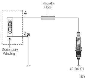
There is an individual ignition circuit and coil for each cylinder on the ME 9.2 system. The ME 9.2 uses "pencil type" ignition coils manufactured by Bremi. The eight individual ignition coils are integrated with the insulated connector (boot).
